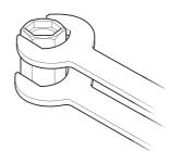
Hold a wrench across the flats of the plastic connector. Unscrew the Filter using another wrench as shown. Clean or renew the Filter as necessary. Refit in reverse order, making sure the Filter is screwed fully home. **Do not** overtighten. Make sure plumbing connections are sealed before restoring electricity supply.
