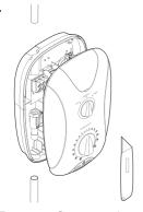
Remove Cover and determine supply pipe position.
