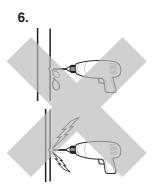
CAUTION! Do not drill into buried cables or pipes.
