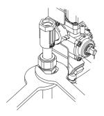
Connect supply pipe. **Do not overtighten!**
