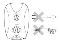
**Do not** use alternative screws to secure the Cover. This can cause internal damage to the appliance. **Do not** seal around the back of appliance.
