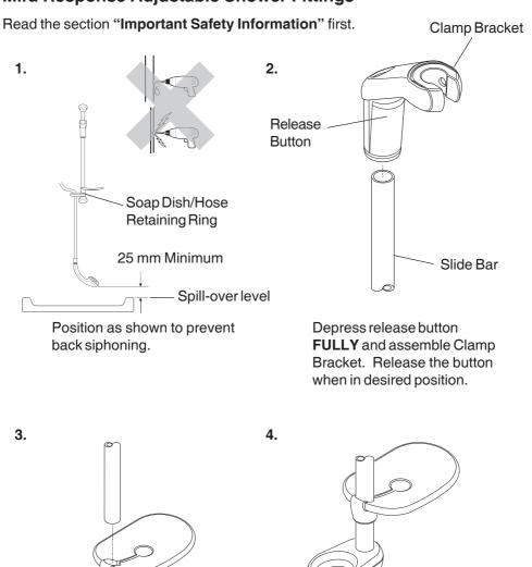
Slide the Soap Dish and the Hose Retaining Ring onto the Slide Bar below the Clamp Bracket. Fit both the top and bottom Supports. Make sure the slots are aligned to fit fully home. 5.
