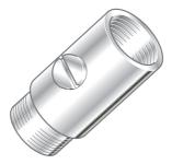
DCV-H: An outlet double checkvalve, designed to prevent the backflow or backsiphoning of potentially contaminated water, through shower controls which are fitted with a flexible hose as part of the outlet shower fitting. Available as an optional accessory from all Mira Showers stockists.
