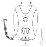
Refit the Service Tunnel and Cover. Make sure they fit correctly. **Do not** overtighten screws. 11.
