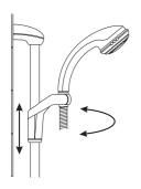
Depress the release button and slide the Clamp Bracket assembly to the required position.
