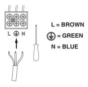
Firmly connect the conductors. **Do not** exert strain on the terminal block.
