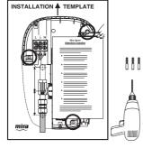
Drill and plug\* the three holes using template.
