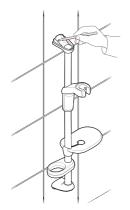
Mark the positions of the slots on both top and bottom Supports.
